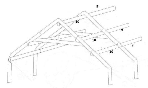
F. Insert leg No.1 and No.3 to the corner arch No. 7 and No.12 as below picture shows .And connect them by cross bar no.10 and no.9 with screws (M8x120mm). No. 9 is for add-on sections . Also at this point, use diagonal 3 to make the frame stable.
