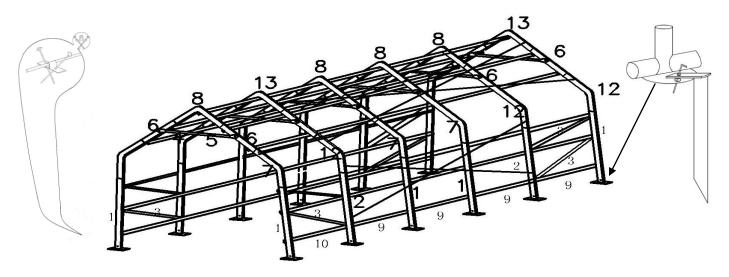
To Spread the cover over the frame. Please pay attention to all sharp edges and potential harm to the cover. Insert pipe No.11 into the bucket at the bottom of the roof .Fasten it with strap,like below picture. Fasten the roof to the structure and by fix it ground with tie down kit .
