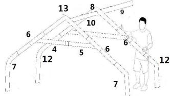
E. Connect the corner arch by cross bar pipe no. 10 and no. 9 with screw (M8x120mm). Still , no. 9 is for add-on sections .
