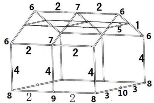
**II** Attach one end of the support poles (4) to the roof joints (6,7).
